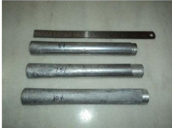
Fig. 1: Al-SiC-Gr hybrid composite specimens with 5%, 7.5% and 10% of SiC-Gr particles
